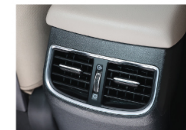
Rear AC Vent
