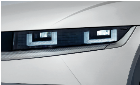
Full LED Headlamps (Projection Type)
