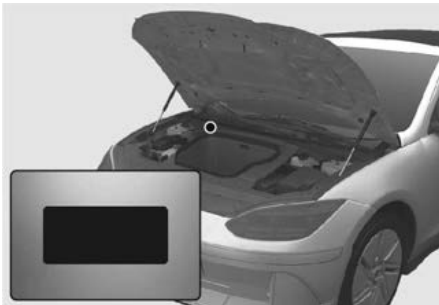
Air Conditioning refrigerant label
